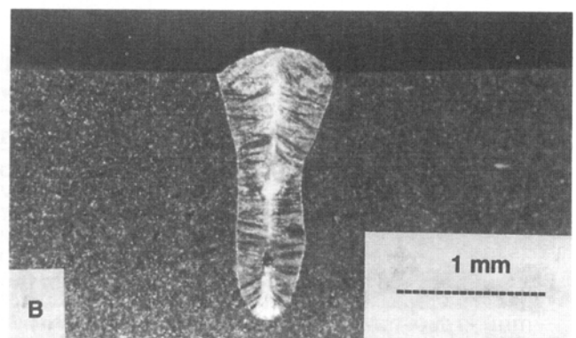
Fig. 11 Laser beam bead-on-plate welds for (a) 304LS, (b) 304HS, and (c) 304C, using argon gas
